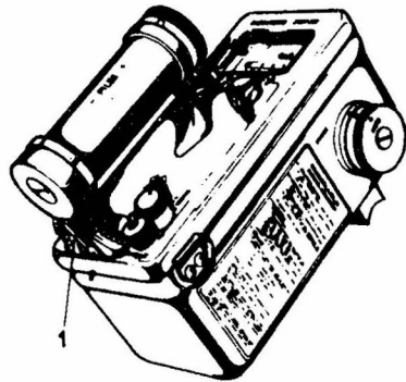
Fig. 17 CHECKING THE DOM 410 RADIATION METER FOR OPERATION ON 10 mR/H RANGE
